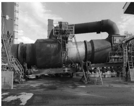
(a) Parallel flow drum mixer was used to produce the mix. The drum was estimated to be 12 years old. The drum was powered by natural gas and was observed in a good condition
