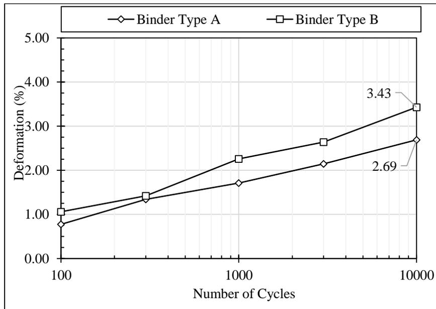
**Figure 2. French Rutting Test Results**
